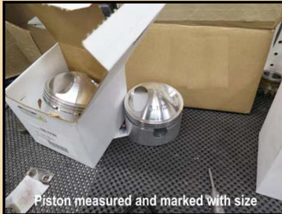
Piston measured and marked with size
