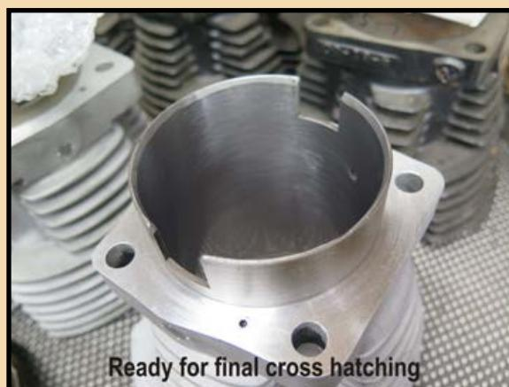
Ring manufacturers state what type of surface finish they prefer. This has all sorts of specs that most DIY folks can't measure – so we'll focus instead on grit. For most rings, 180-220 grit finishing stones are perfect. The easiest way for DIY folks to achieve a good surface finish is with a ball hone. Choose your size and grit – and have at it
