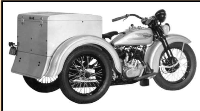
The Servi-Car was designed in the early part of the Great Depression for the conditions of its day, in which roads might be crude and unpaved. It has a rigid rear axle with a differential. The rear axle has a track of 42 inches (1,100 mm), similar to the track of most cars at the time. This allowed it to follow ruts that had already been worn into the road.
